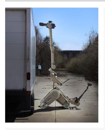
Kobra 725 provides unmatched strength, power, and payload support. The robot is designed to be a remote operational platform with a manipulator arm capable of lifting heavy loads. Kobra 725 is highly maneuverable in rough terrain and able to climb stairs. The state-ofthe-art, IOP-compliant system allows for future payload expansion. Kobra 725 allows easy integration and deployment of a large range of accessories for EOD, CBRN/HazMat, breaching, and other applications.
